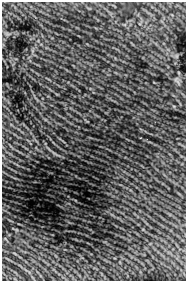
FIGURE 4 Smectic ( S_3 ) schlieren texture exhibiting gridlike pattern with domain walls manifested from undulation line 4O(OH)_6 at 70^\circ C .
