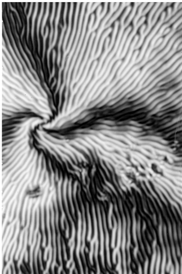
FIGURE 1 Smectic schlieren texture with undulation line 4O(OH).6 at 60°C.
