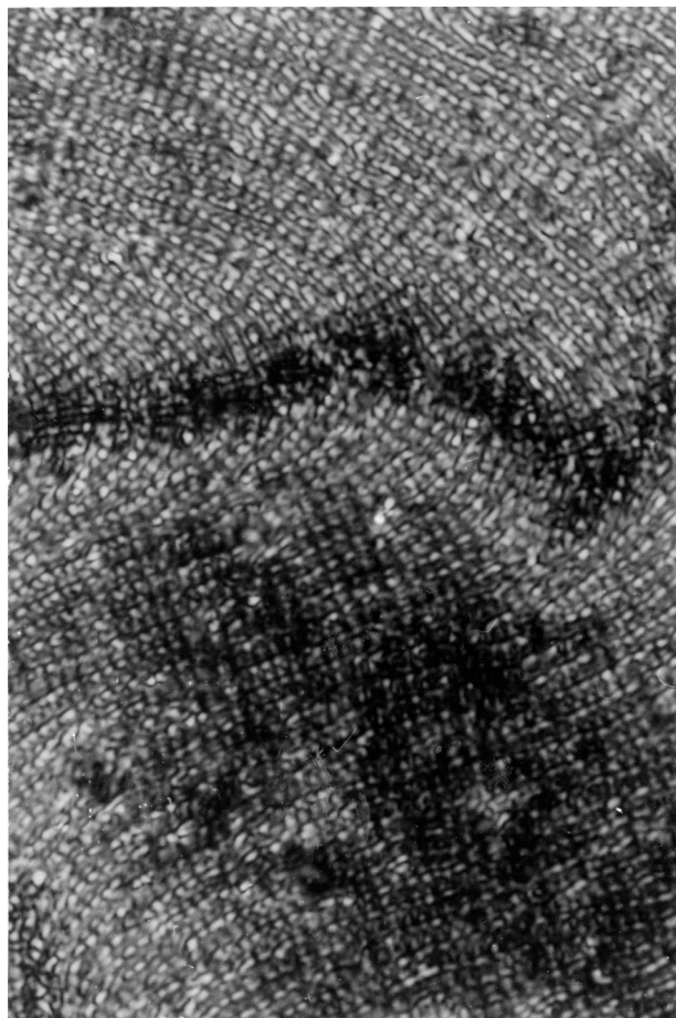
FIGURE 3 Smectic C schlieren texture with crosshatched pattern manifested from double undulation line 4Q(OH)_6 at 75^\circ\text{C} .
